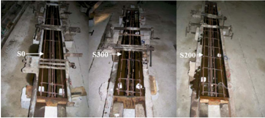
Fig. 3.5 Cages of RC T-beams before casting for series S0, S300 and S200
